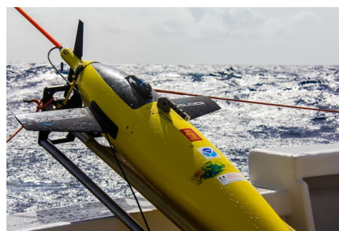
Underwater hurricane glider. Credit: NOAA
