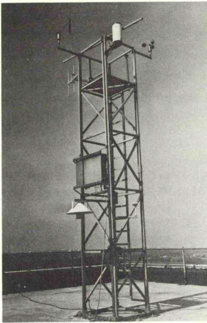
Automatic weather stations provide surface meteorological data from remote or unmanned locations.
