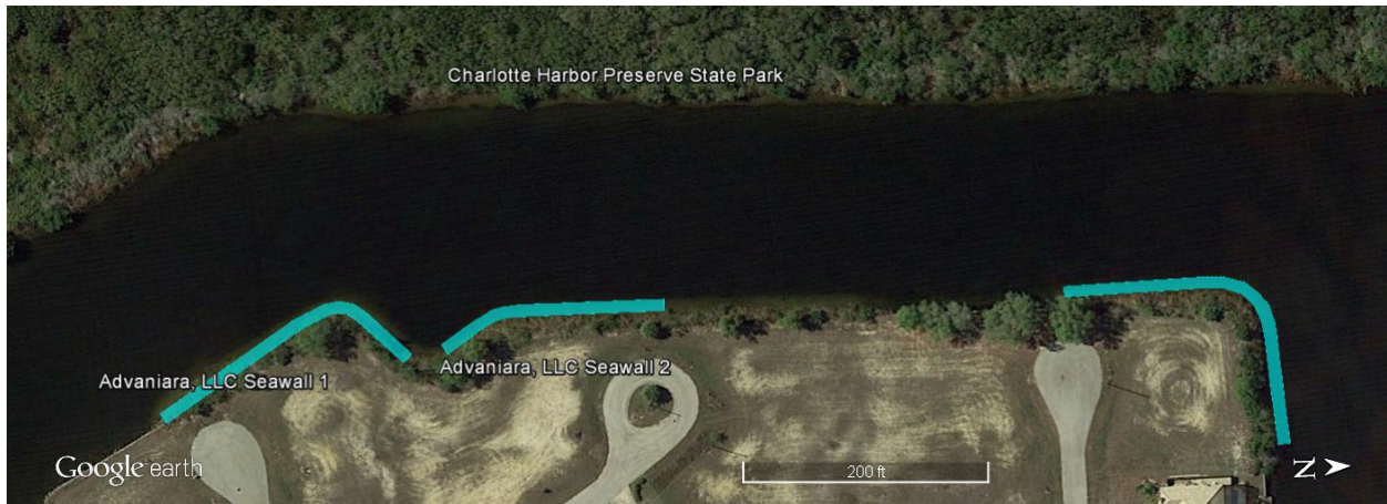
Figure 1. Image showing the approximate locations of the 3 proposed action areas and their proximity to the Charlotte Harbor Preserve State Park, which includes the mangroves shown at the top of the image; the approximate action areas are depicted in light blue, and assume deployment of turbidity curtains approximately 10-ft waterward of the shoreline (©2017 Google)
