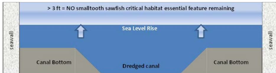
Figure 4. Diagram A depicts a cross section of a historically dredged channel/canal within the boundaries of the critical habitat units that has not been maintained. Diagram B depicts the typical cross section of a maintenance dredged channel/canal. Diagram C depicts a cross section of a maintained dredged channel/canal after sea level rise of > 1 ft.
