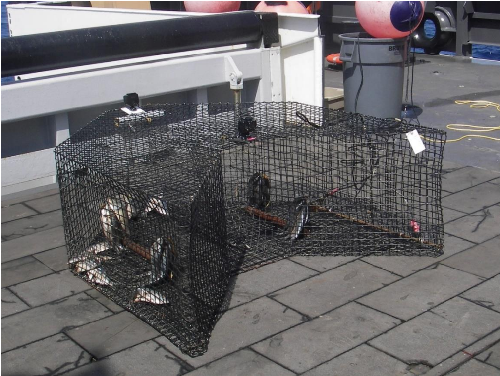
Figure 1. Chevron trap with video cameras used to sample reef fish on the PC-21-03 survey.
