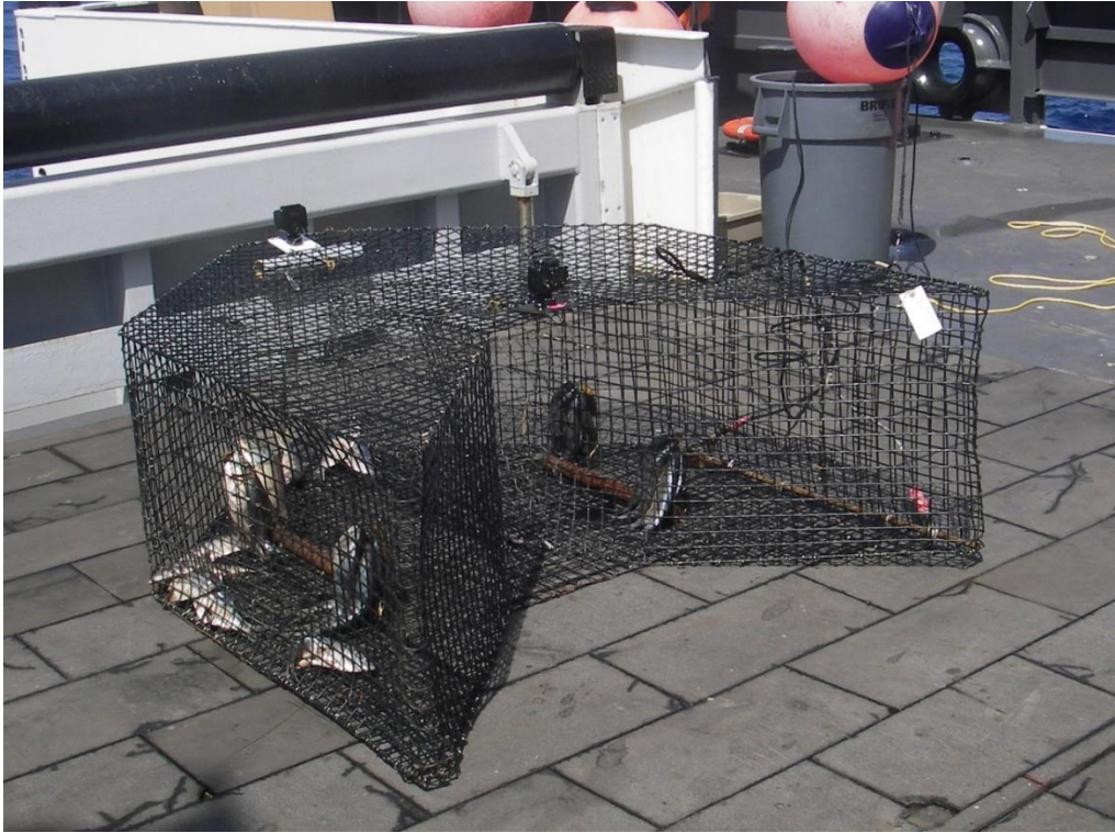
Figure 1. Chevron trap with video cameras used to sample reef fish on the PC-19-03 survey.
