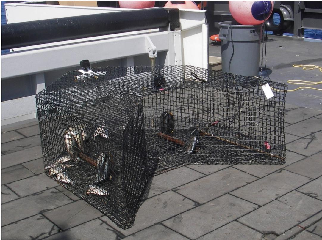
Figure 1. Chevron trap with video cameras used to sample reef fish on the PC-17-03 survey.
