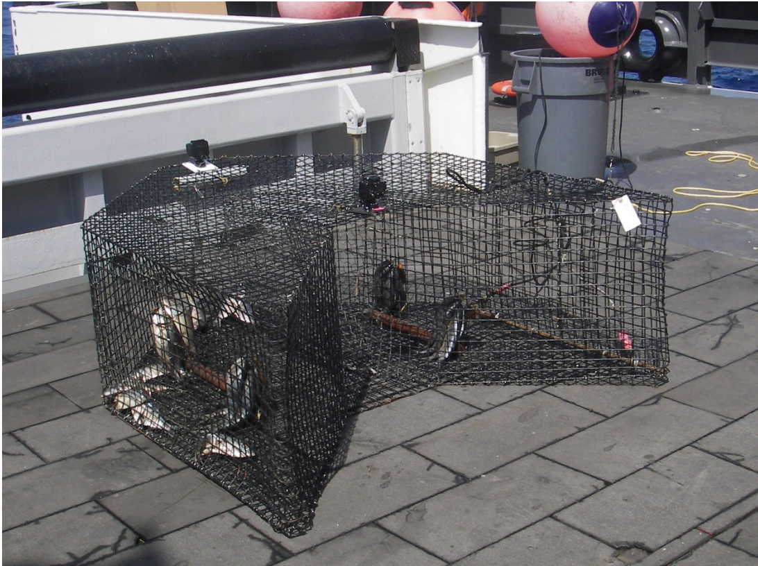
Figure 1. Chevron trap with video cameras used to sample reef fish on the PC-16-03 survey.
