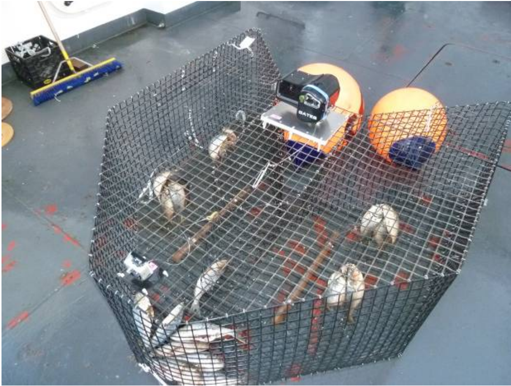
Figure 1. Chevron trap with video camera gear used to sample reef fish on the PC-13-04 survey.
