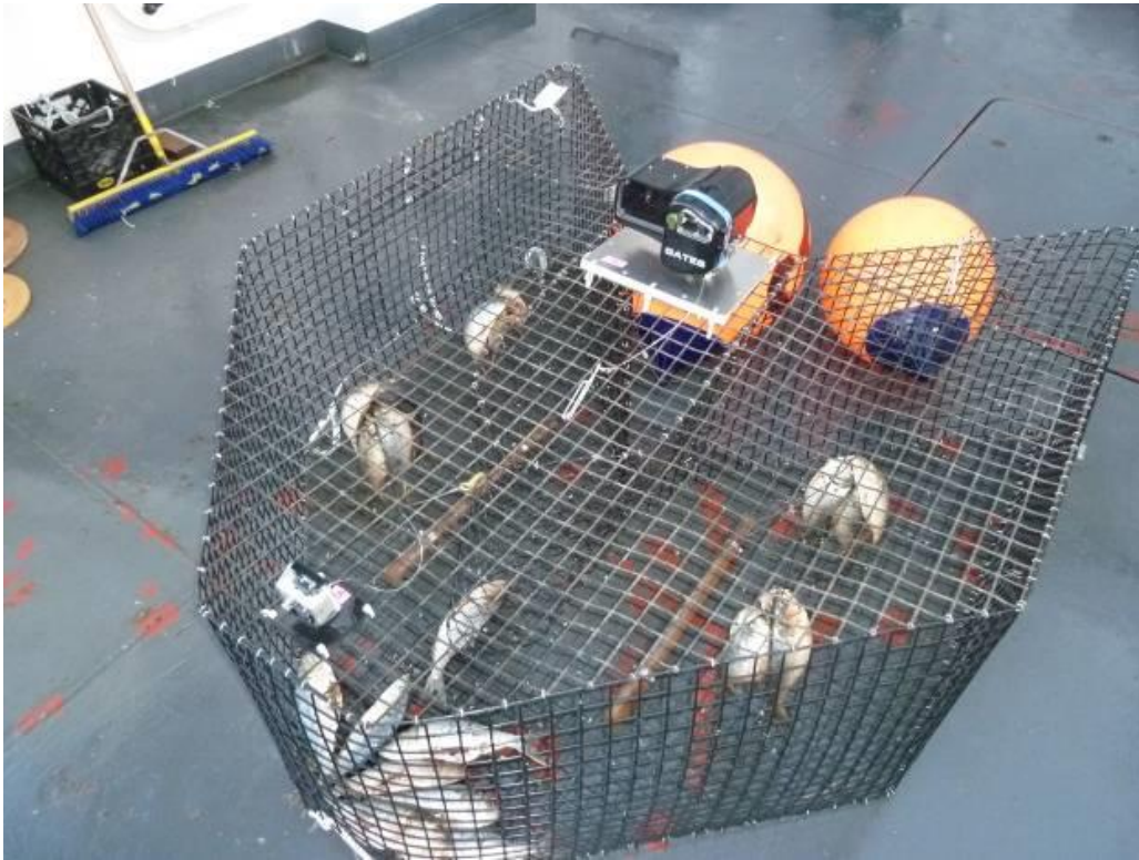
Figure 1. Chevron trap with video camera gear used to sample reef fish on the PC-12-04 survey.
