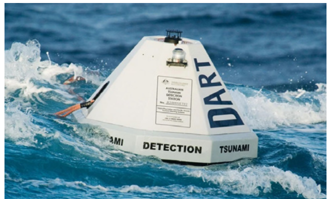
DART buoys detect tsunami waves and transmit real-time sea level information measurements back to the Tsunami Warning Centers. Credit: NOAA
