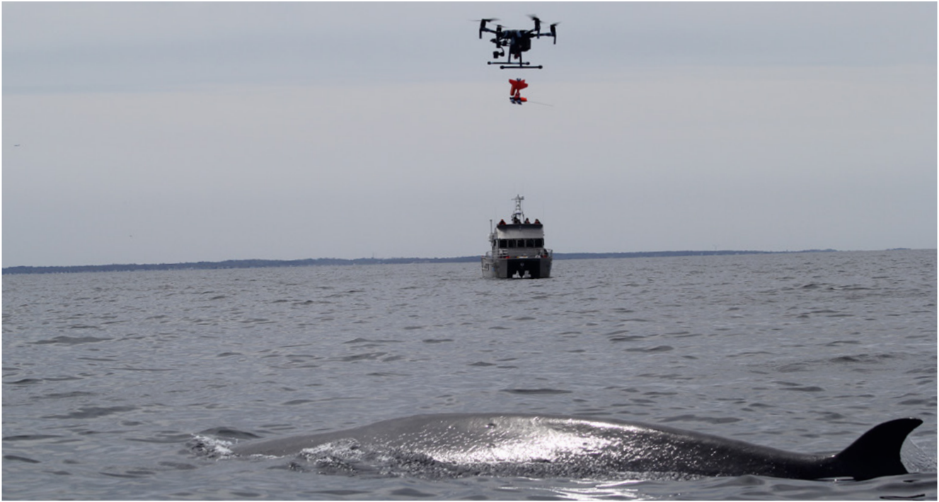
An uncrewed aerial system (UAS) attaches a suction-cup equipped synchronous motion, acoustic recording tag (DTAG) to a sei whale. This is the first time a UAS was used to tag sei whales and the first use of a UAS to tag free-swimming large whales in U.S. waters. Photo taken under NOAA Fisheries Permit No. 18786-06. Photo credit: Laura Howes
