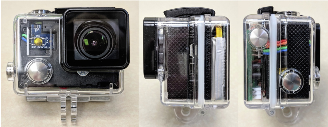
Fig. 1. A fully assembled CoralCam unit consisting of the modified camera, CoralCam PCB assembly, and microcontroller battery fitted into a GoPro Hero 4 underwater housing with “extended back door”.
