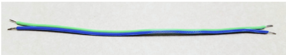
Fig. 5. Example of an approximately 10 cm paired wire consisting of two individual wires. One paired wire will be connected to the camera Mode/Power button and one to the camera Shutter button.
