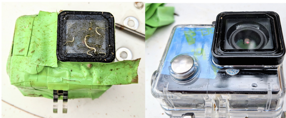
Fig. 19. (left) A CoralCam with biofouling immediately following 30 days of deployment, (right) and after removal of the electrical tape wrapping and gentle scrubbing of the front lens.
