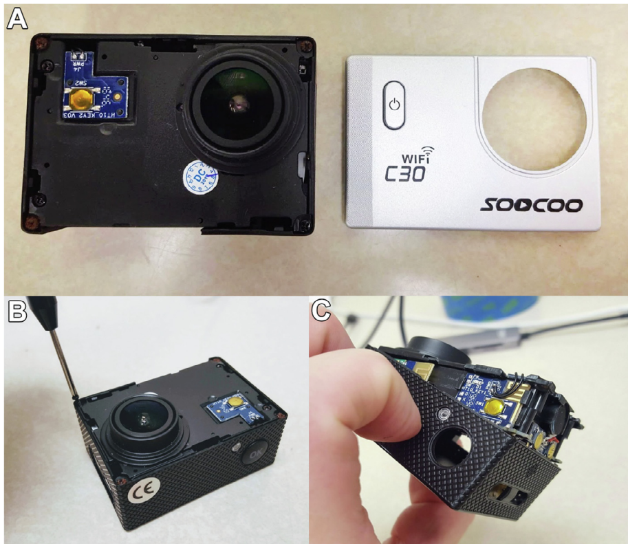
Fig. 4. (a) The camera to be modified with face plate removed, (b) during removal of frame screws, and (c) after partial separation of the camera frame from camera assembly.
