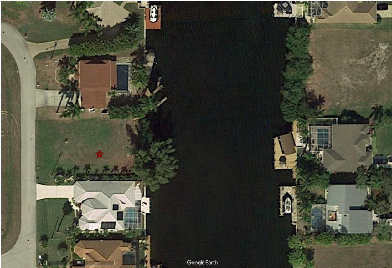
Figure 2. The project site at 5307 Southwest 26th Court, Cape Coral, Lee County, Florida, along Palos Canal, showing 80 lin ft of unconsolidated shoreline (©2018 Google).
