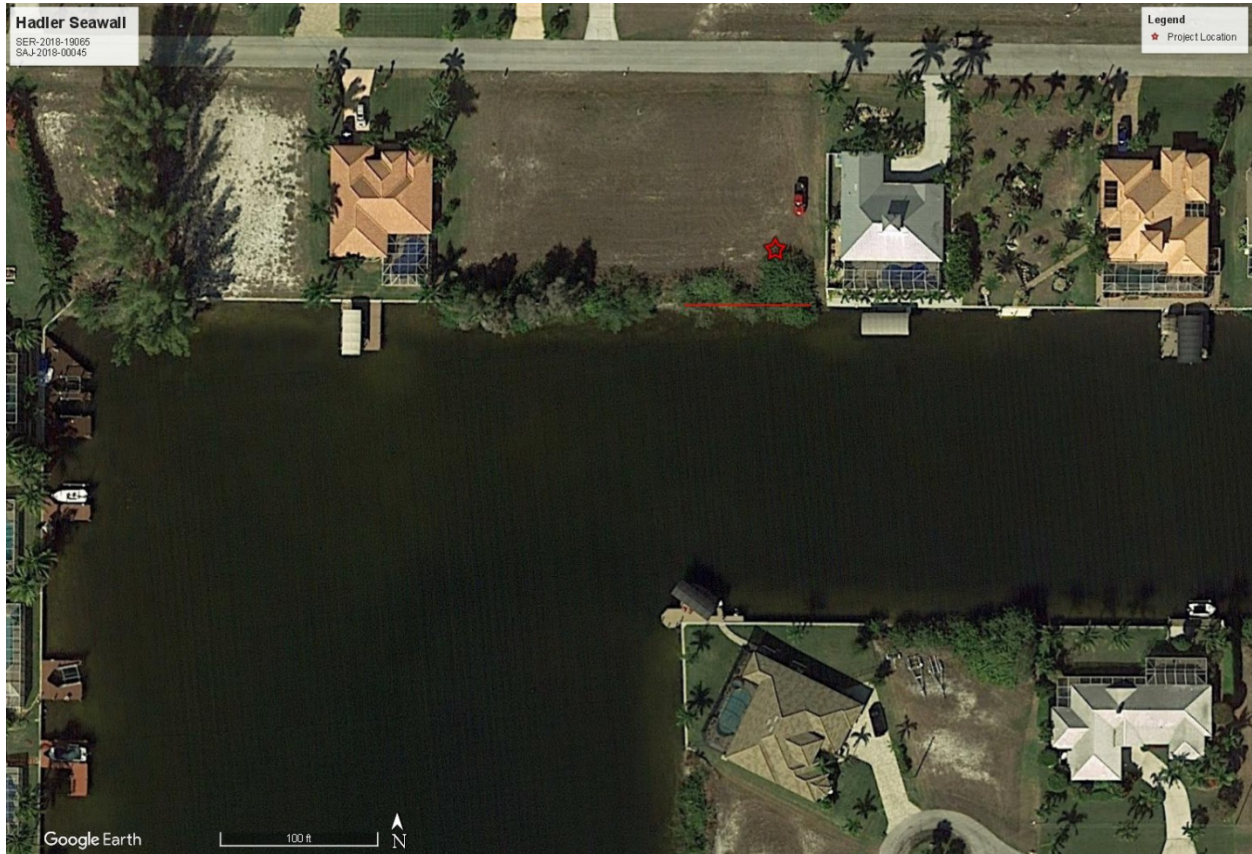
Figure 2. The project site at 4118 Northwest 11th Terrace in Cape Coral, Lee County, Florida, and similar habitat nearby. The red line indicates the 80 linear feet (lin ft) of unconsolidated shoreline under consideration in this project (©2018 Google).
