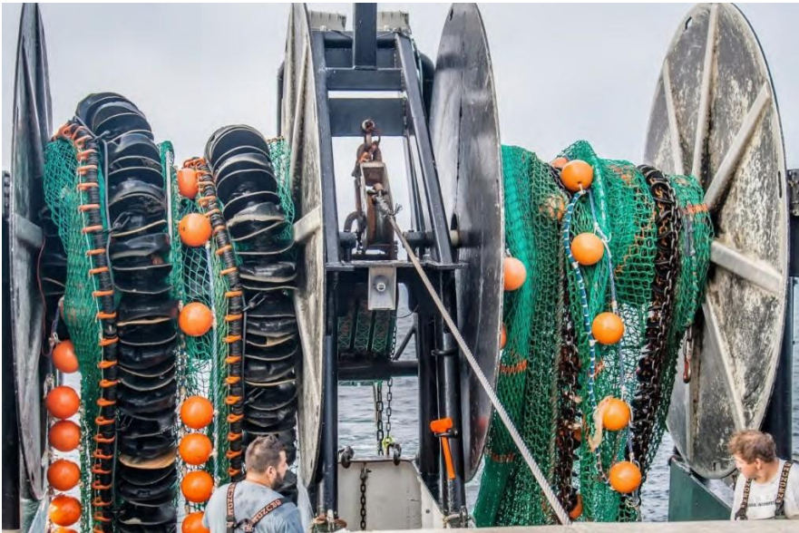
Figure 4.8. Image of the rockhopper and chain sweeps on the F/V/ Karen Elizabeth.
