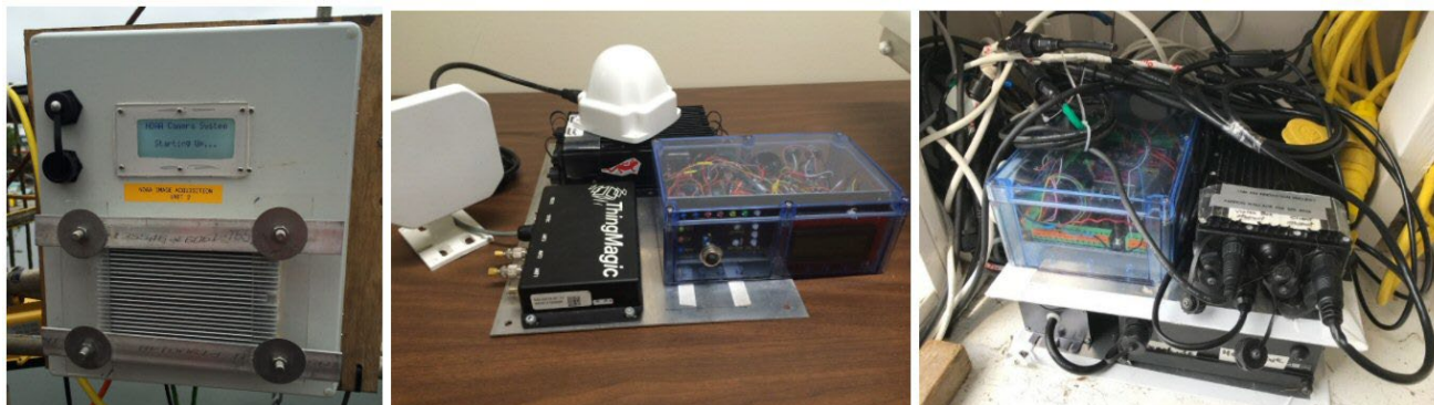
Figure 6. -- EM Rail system hardware evolution. Left image depicts initial design with right image being the most recent deployed version.
