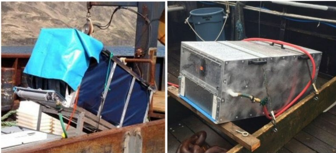
Figure 34. -- Evolution of the physical chute design showing the design improvement from the early MV camera chute (left) to the halibut bycatch chute design (right).
