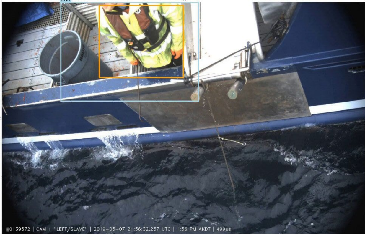
Figure 55. -- Image frame from an example of Crew on Deck detection. The light blue bounding box is the ROI with orange bounding box being the detection.
