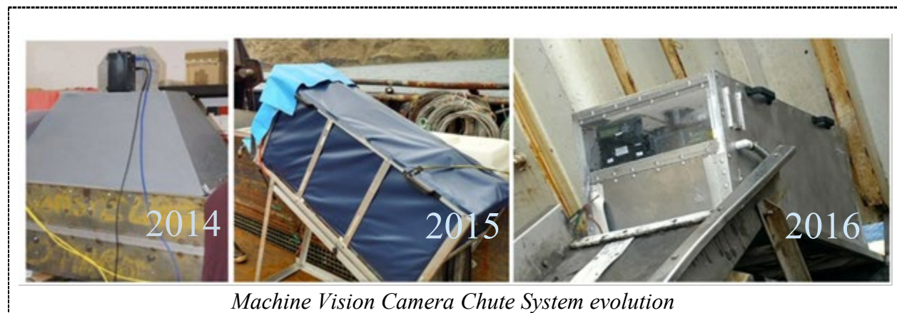
Figure 23. -- MV camera chute (MVChute) systems design, showing the progressive design evolution (upper three panels).
