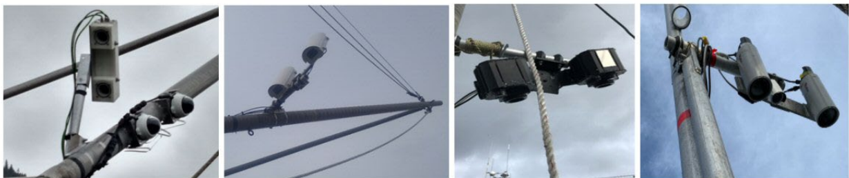
Figure 4. -- Evolution of stereo camera housing design with the left-most photo showing the initial camera housing through to the current housing design.
