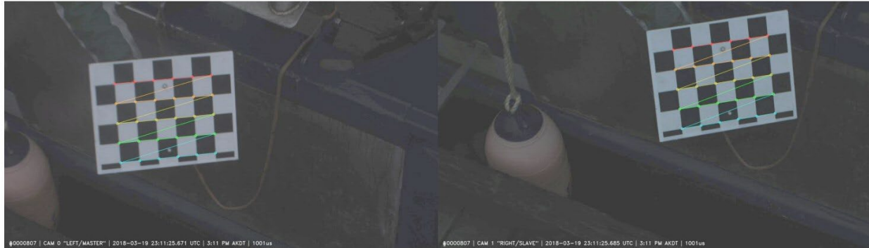
Figure 10. -- An example of the checkerboard used in calibration of the stereo Rail system.
