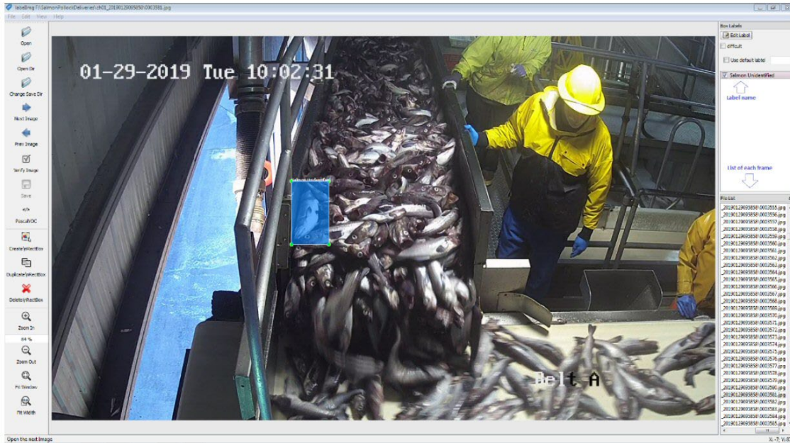
Figure 50. -- Photo extracted from video recording of a pollock delivery in a shoreside processing plant. The bounding box in the center of the image (shaded blue) shows an annotated salmon detection.
