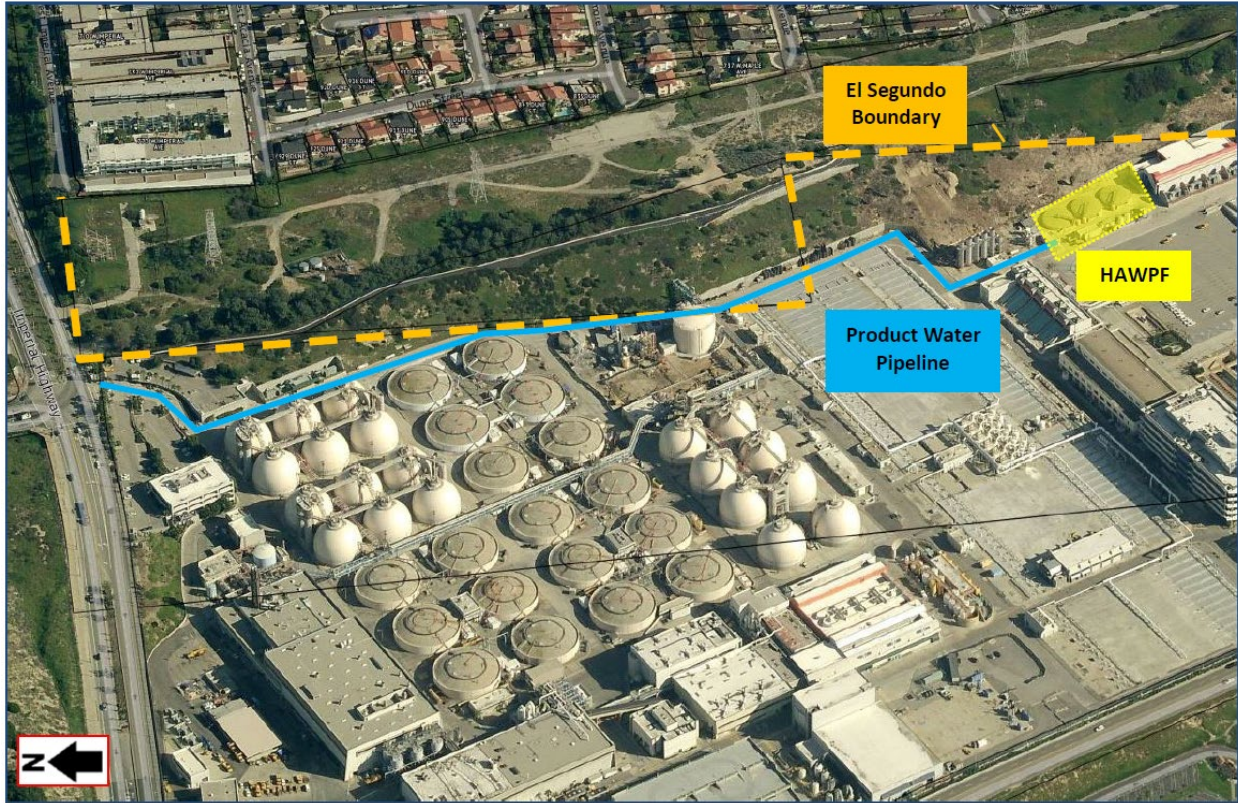
Figure 2. Location of the Advanced Water Purification Facility inside Hyperion. (LA Sanitation and Environment 2021).
