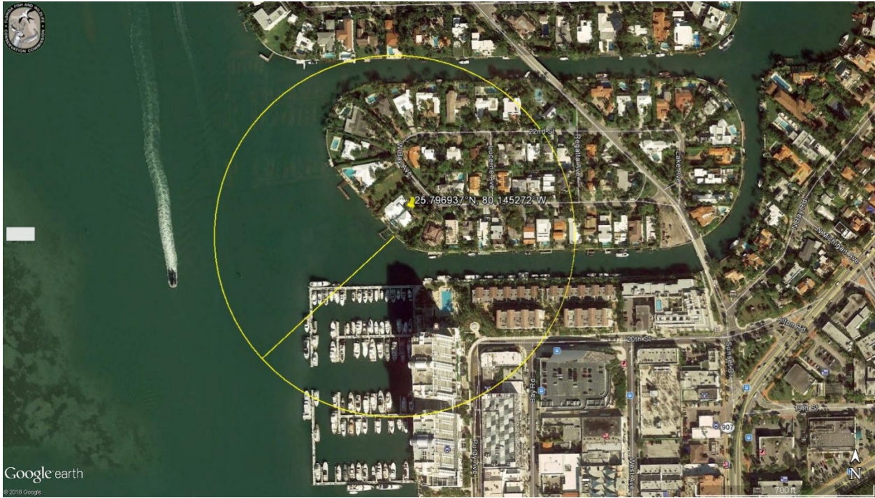
Figure 3. Image showing the action area defined by the extent of behavioral noise effects based on the proposed action’s installation of 12-in wooden piles using impact hammer (©2018 Google).
