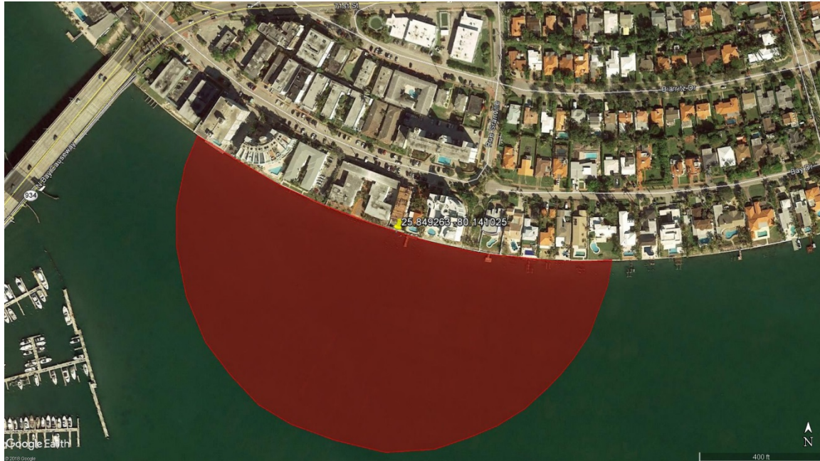
Figure 3. Image showing the action area defined by the extent of behavioral noise effects based on the proposed action’s installation of 12-inch concrete piles using impact hammer (©2018 Google).
