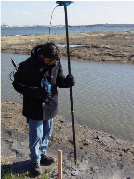
Figure 14. Post-construction Real-Time Kinematic (RTK) GPS survey at Ft. McHenry Wetland.
