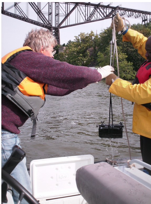
Figure 6. Drs. Lowenstein (left) and Apeti (right) retrieving a Ponar sediment grab (Credit: NOAA).
