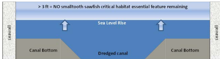
Figure 5. Diagram A depicts a cross section of a historically dredged channel/canal within the boundaries of the critical habitat units that has not been maintained. Diagram B depicts the typical cross section of a maintenance-dredged channel/canal. Diagram C depicts a cross section of a maintained dredged channel/canal after sea level rise of > 1 ft.
