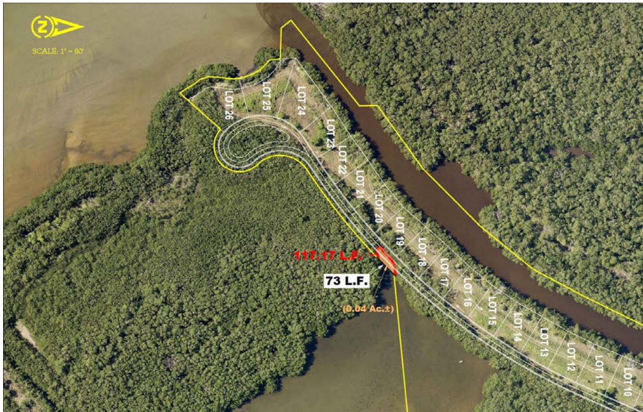
Figure 5. Location of the portion of the proposed action occurring waterward of MHW along the east side of Lot 18 and Lot 19. The 117.17 lin ft of red mangroves to be removed and replaced by 73 lin ft of riprap is outlined in red. The 0.04 ac of shallow water habitat to be filled is highlighted in orange (Image provided by USACE).
