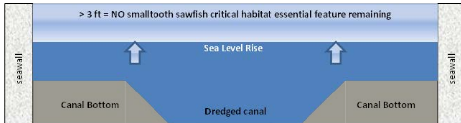
Figure 8. Diagram A depicts a cross section of a historically dredged channel/canal within the boundaries of the critical habitat units that has not been maintained. Diagram B depicts the typical cross section of a maintenance dredged channel/canal. Diagram C depicts a cross section of a maintained dredged channel/canal after sea level rise of > 1 ft.
