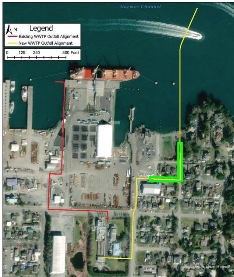
Figure 2. Overhead photograph of the project site on the northeast corner of Anacortes, Washington. The existing outfall route is shown in red the proposed new outfall route is shown in yellow (both extending from the City's wastewater treatment plant). The planned upland blasting area is outlined in bright green (Adapted from Figure 2 in Widener 2021a, and Figure 8 in McMillen Jacobs 2022).
