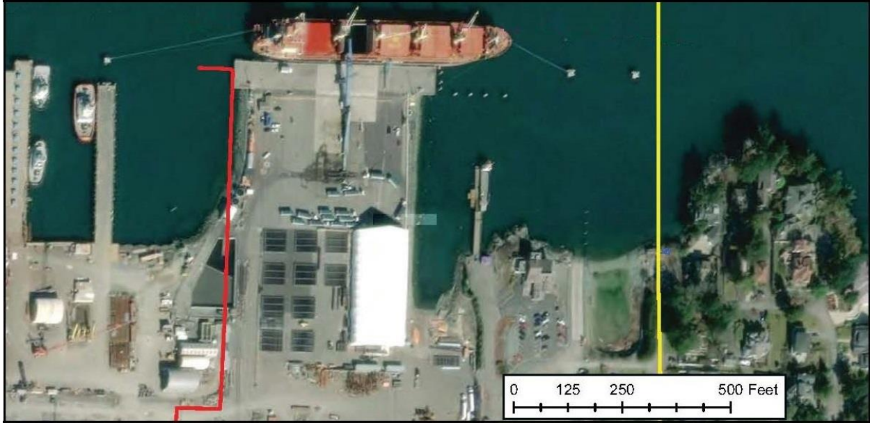
Figure 11. Overhead photograph of the shoreline portion of the project area at the north end of Anacortes, Washington. The yellow line indicates where the proposed replacement pipeline would cross the shoreline. The existing outfall pipeline route is shown in red, running west of the Port's Pier 2 (Adapted from Figure 2 in Widener 2021a).
