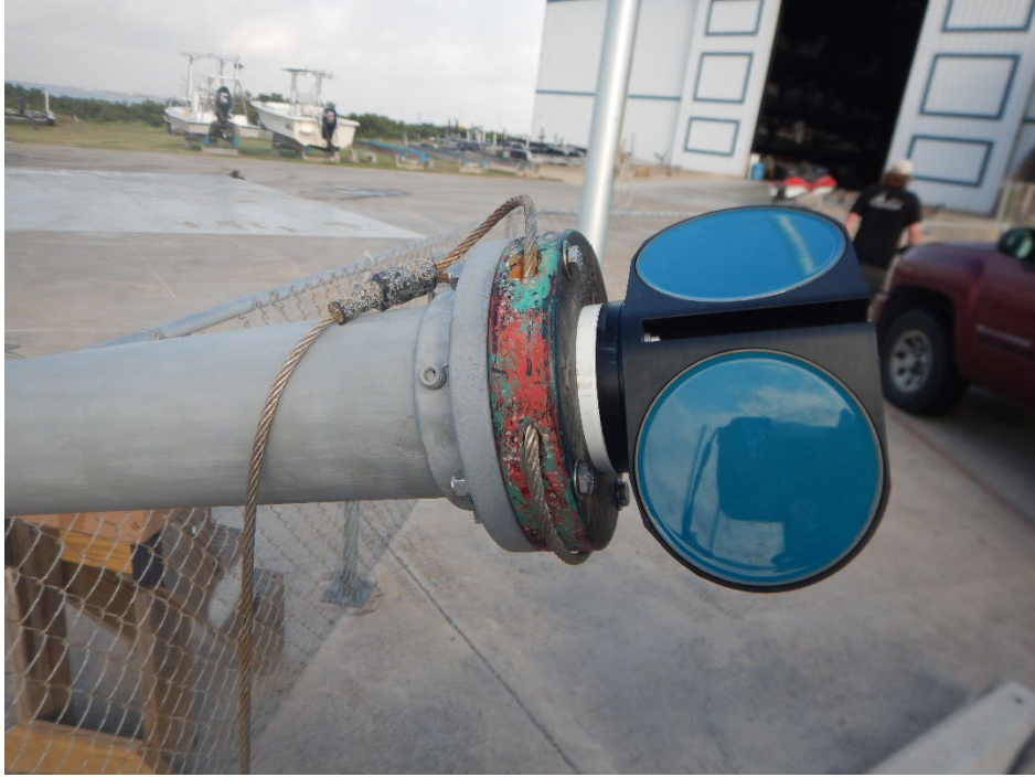
Figure 3-3. Side-looking Nortek Aquadopp ready for installation at the end of the pole to be clamped to a fixed structure.
