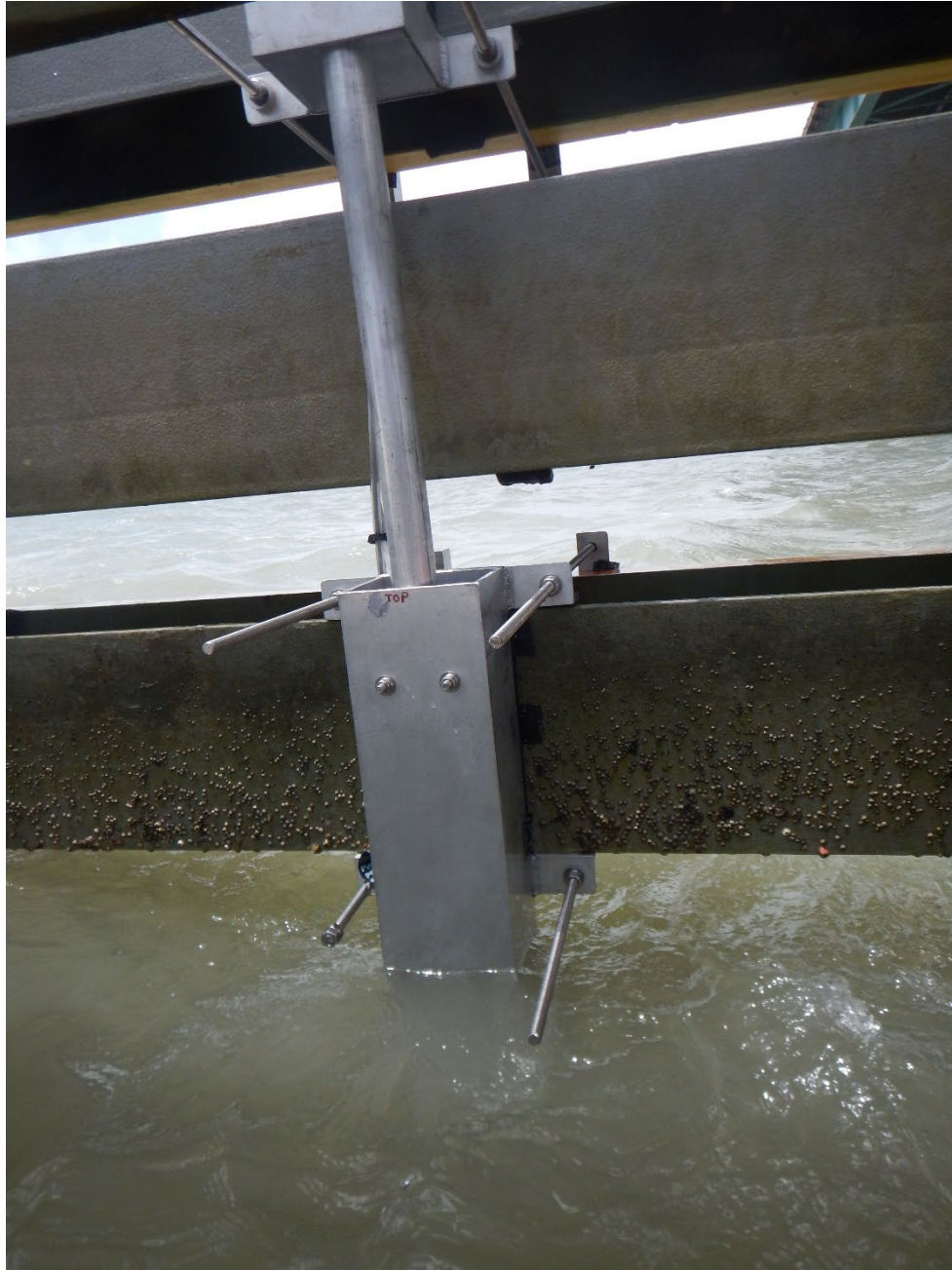
Figure 3-5. Horizontal crib count on the Queen Isabella Bridge. An acoustic Doppler current profiler (ADCP) is held at the bottom of the pole, below the surface.
