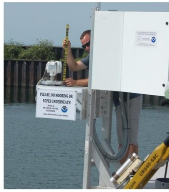
Figure 2. Radar sensor survey collar drawing and field level survey process photos.
