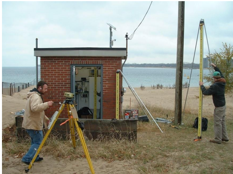
Figure 4. Fort Gratiot, MI, (gauge house atop the concrete well) leveling survey.
