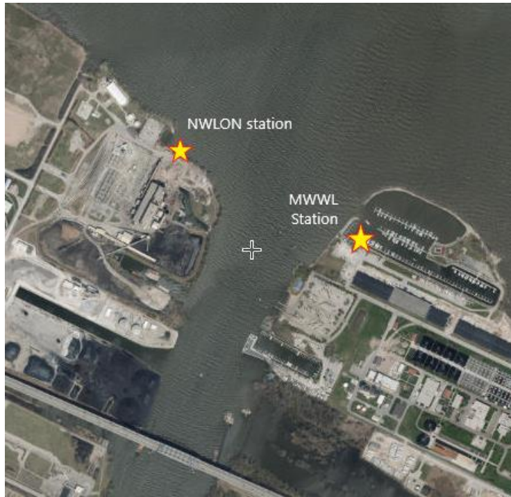
Figure 22. Locations of the original primary National Water Level Observation Network (NWLON) station and the microwave water level (MWWL) station at Green Bay, WI.
