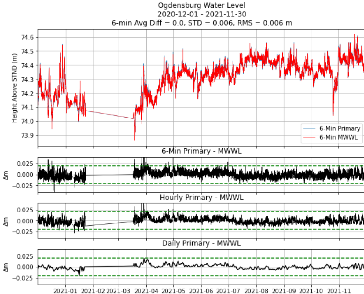
Figure 26. Time series of primary (National Water Level Observation Network [NWLON]) and microwave water level (MWWL) differences for 6-minute, hourly, and daily values at Ogdensburg, NY.
