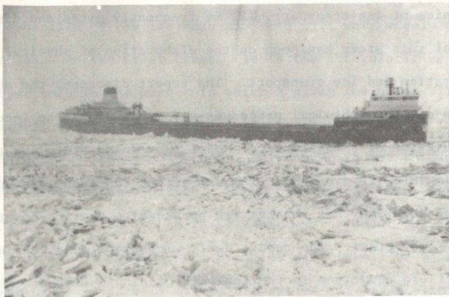
Figure 1.2 The lake ore carrier, Roger Blough, pinned between shore fast grounded ice and drift pack ice near Conneaut, Ohio (Feb. 8, 1979).
