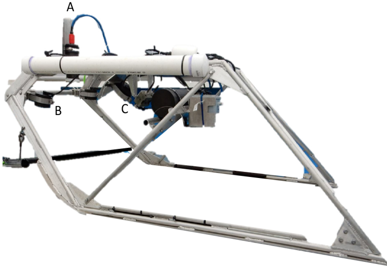
Figure 2. The camera sled main parts include: (A) camera housing, (B) strobe lights, and (C) onboard computer.
