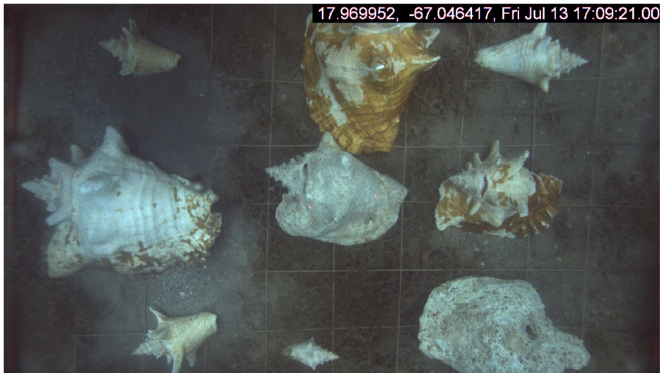
Figure 3. Camera sled laser calibration. Nine conch were distributed in different locations to compare length estimated with the lasers and the caliper. Laser dots in the center of the image are 10 cm apart.
