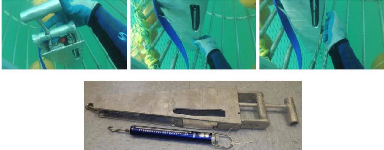
Figure 11. Graduated metal wedge used to allow divers to measure CTED bar spacing.
