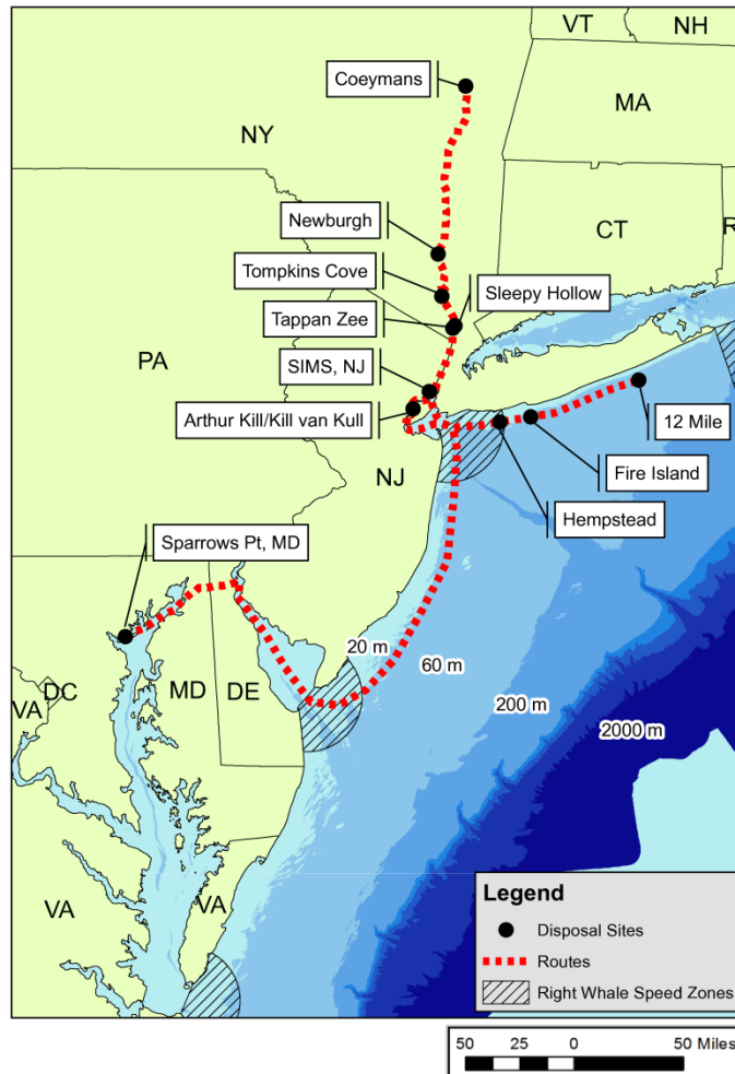
Figure 5. Potential routes to be traveled by project vessels transporting demolition debris from the existing Tappan Zee Bridge to possible disposal sites. Hatched areas indicate seasonal management areas for North Atlantic right whales where a speed restriction of 10 knots or less is in effect for vessels 65 feet in length or greater from November 1 through April 30 (50 CFR 224.104). However, FHWA has indicated that compliance with this restriction will be required for disposal vessels regardless of length.
