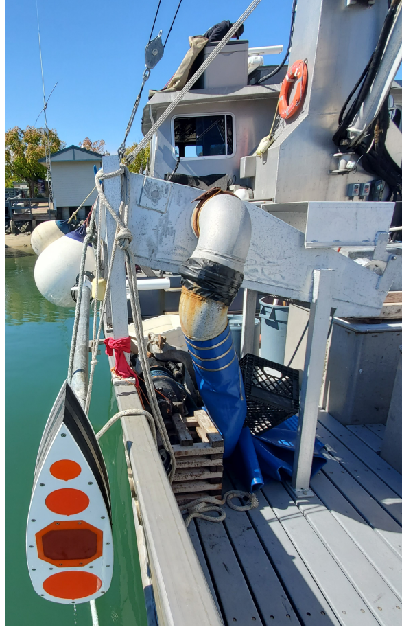
Figure 5: Transducers (Top-bottom: Simrad ES200-7C, ES120-7C, ES38-12, and ES70-7C, Kongsberg) in a pole-mounted multi-transducer array (MTA4) installed on the Long Beach Carnage .
