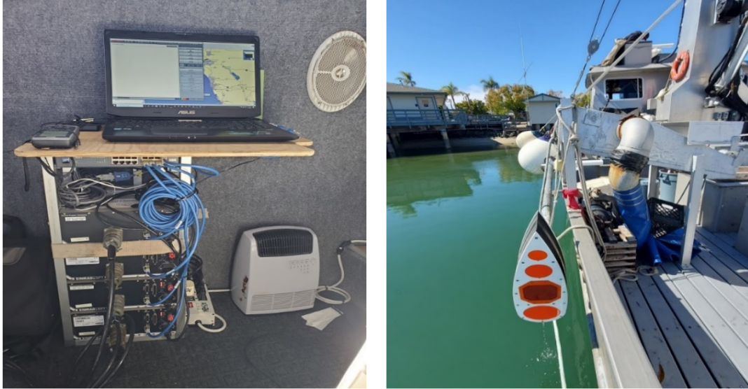
Figure 6: The four-frequency scientific echosounder system aboard F/V Long Beach Carnage included four Simrad EK60 GPTs (Kongsberg; left) and four split-beam transducers with center frequencies of 200, 120, 38 and 70 kHz (Kongsberg; top to bottom; right).
