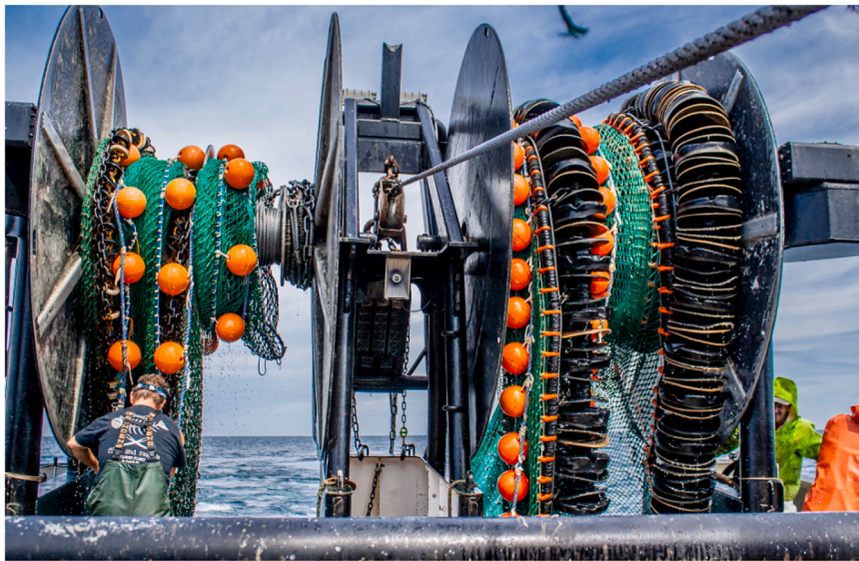
Fig. 2. The F/V Karen Elizabeth twin-trawl vessel rigged with rockhopper sweep gear on the right and chain sweep gear on the left.
