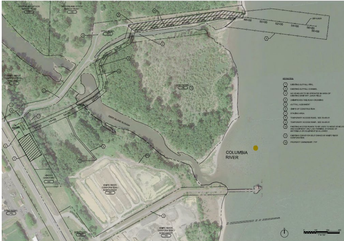
Figure 3. Staging area and temporary road construction.
