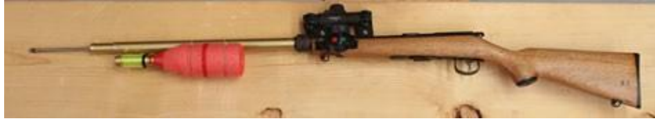
Figure 13. Paxarms large whale custom-made remote sedation system with assembled dart loaded into projector barrel and tether/float attached to barrel. (Photo credit: IFAW)
