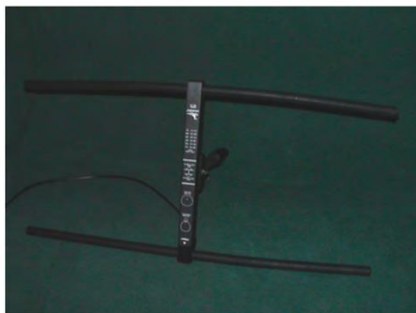
2 – element Yagi antenna
