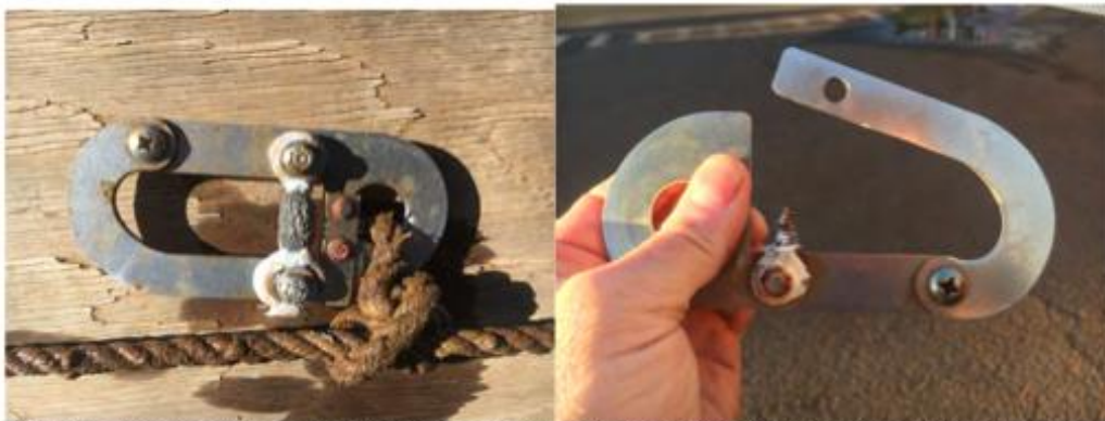
A pitted galvanic release in need of replacement and a spent timed release in need of a new galvanic release. Note the missing hardware on the open clip side.
