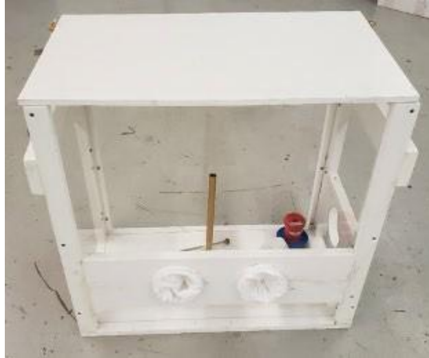
Figure 15. Custom-made splash box for safer at-sea dart loading (photo credit: IFAW)
