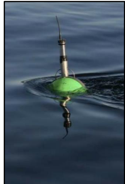
Telemetry buoy with transmitter trailing behind entangled animal (NOAA AKPRD)
