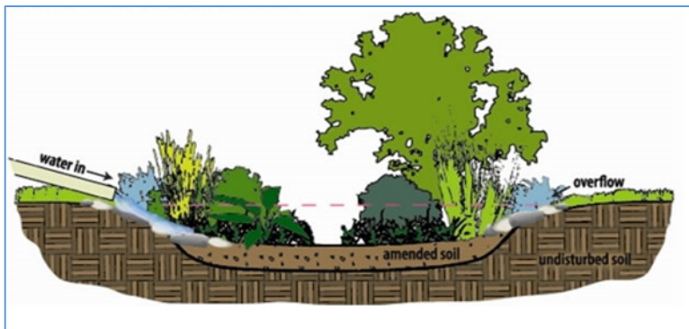
Figure 1. A bioretention cell as an example of green infrastructure in which stormwater runoff enters and infiltrates into the ground through the amended soil rather than into a storm drain. (Source: EPA, 2018 )
