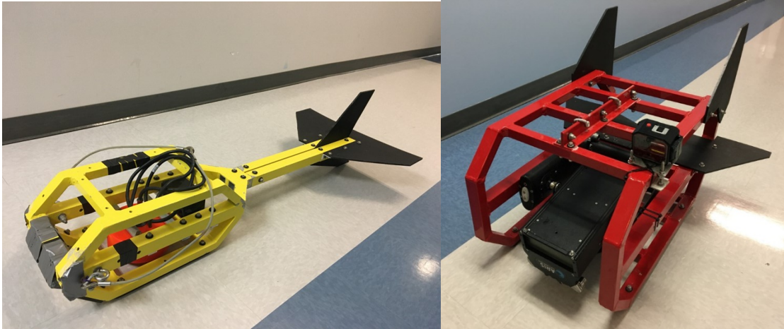
Figure 15. Tow body for the echosounder transducer (orange cylinder at frame center), and video collection tow body for the imaging sonar unit and the standard cameras.
