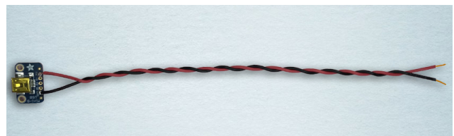
Figure 26. 5-volt power supply that connects to (+) and (-) sockets on the protoboard
