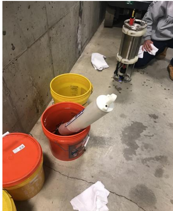
Figure 5: Salinity and Temperature verification with Midas CTD+ [3] and Seabird 16 CTD.
