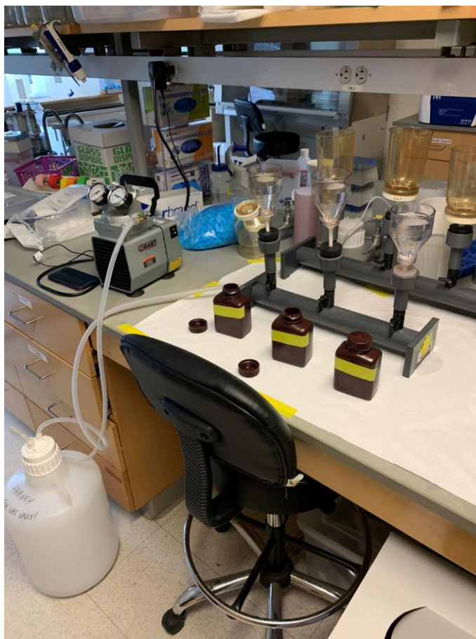
Figure 9. Processing of water samples collected from the Memorial Bridge platform in Portsmouth, New Hampshire. The Acetone filtration process is being performed in the Harvey Laboratory to extract Chlorophyll-a.
