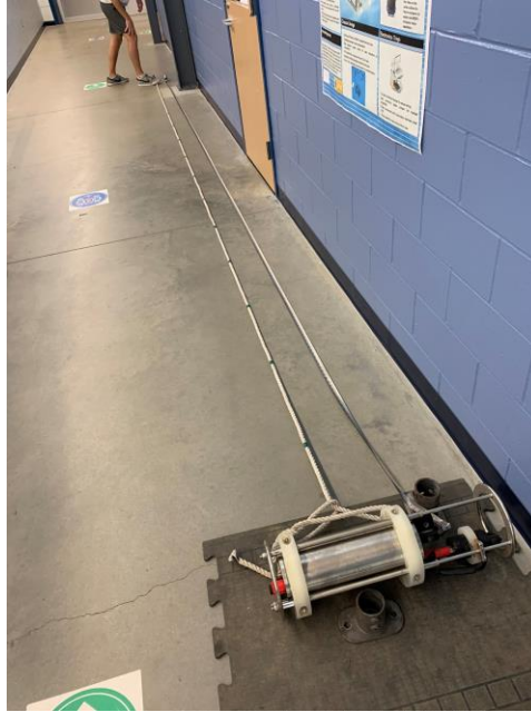
Figure 4: Process of measuring a rope in half meter increments for pressure sensor verification.
