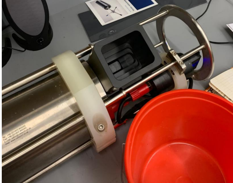
Figure 6: Start of Seapoint STM turbidity sensor verification with the plastic calibration pot snug around the sensor.
