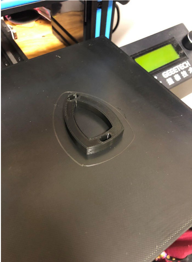
figure 12: First rib of Robo-Fish printed in PLA.
