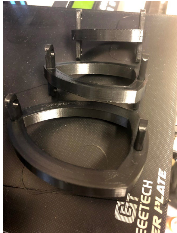
figure 13: All three ribs of the initial Robo-Fish tail printed in PLA with the connectors.
