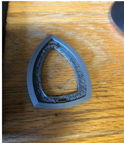
figure 11: A failed print using PETG.
