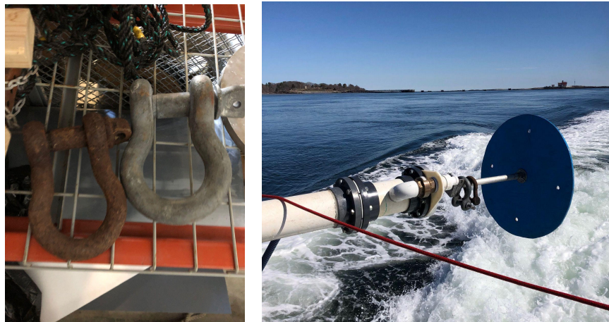
Figure 11a (left): The two shackles used for ballasting during field testing. Figure 11b (right): The two shackles looped around the heave plate pipe after the field test was conducted
