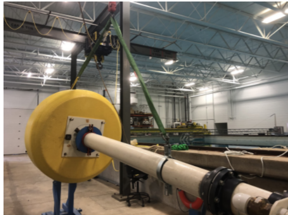
Figure 17: The WPWP being lifted in the UNH High Bay with the final strap lengths and clamp location.
