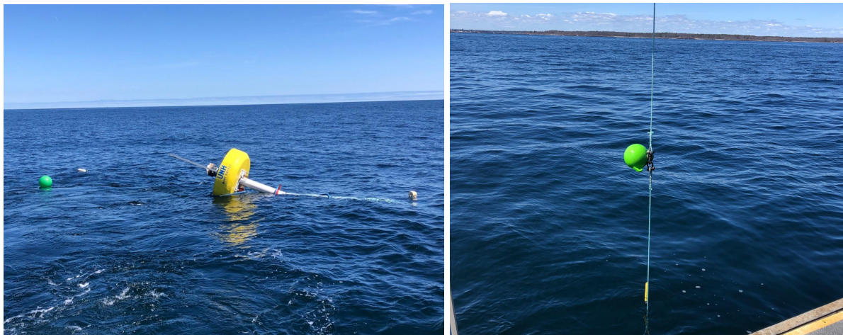
Figure 29a (left): The WPWP initially resting on its side when first deployed
