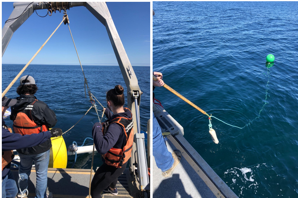
Figure 28a (left): Dakota pulling on the quick release to deploy the WPWP Figure 28b (right): John Ahern hooking the tagline to connect the WPWP to the green surface buoy.
