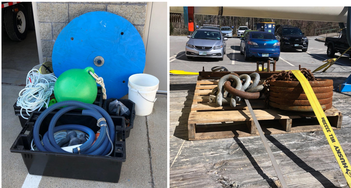
Figure 25a (left): All the mooring lines, floats, heave plate, etc. to be loaded onto the CCOM truck.
