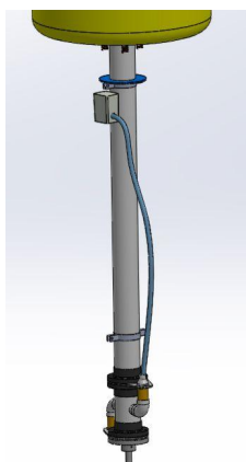
Figure 19: Solidworks modeling of the outlet tube and the flow sensor attached right below the lower stopper.
