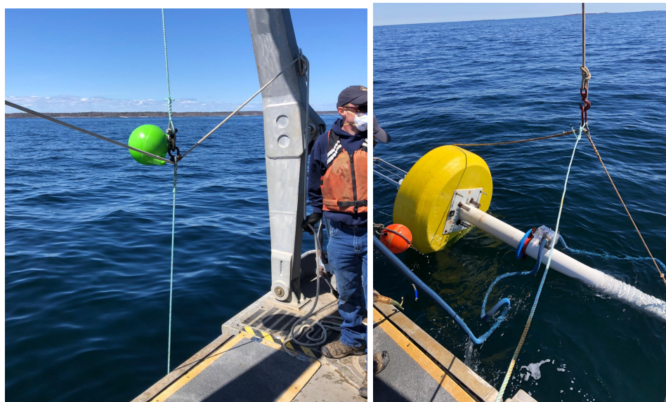
Figure 31a (left): The horizontal rope across the A-frame allowing for the winch rope to be transitioned to the main line.
