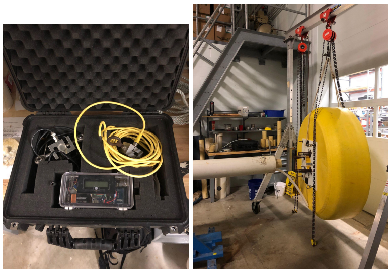
Figure 21a (left): The load cell used to weigh the spar, float, and tee housing
