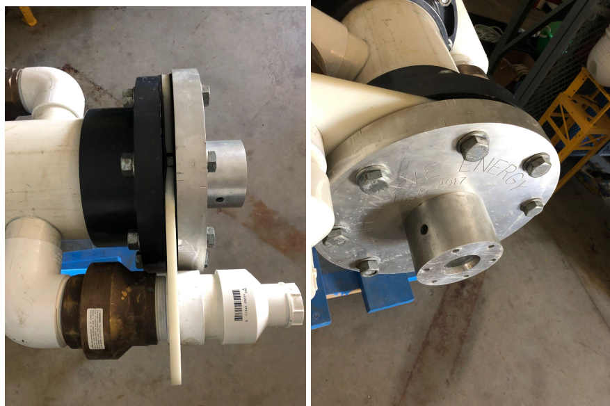
Figure 10a (left): The lower acrylic guide plate sandwiched in between the lower flange and the metal plate for heave plate attachment, supporting just below the check valve
