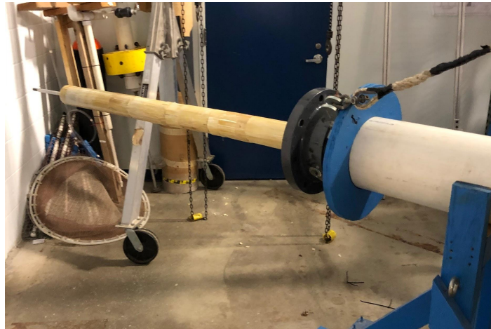
Figure 13: The foam on the piston shaft, cut into small pieces to slide into the piston cylinder.
