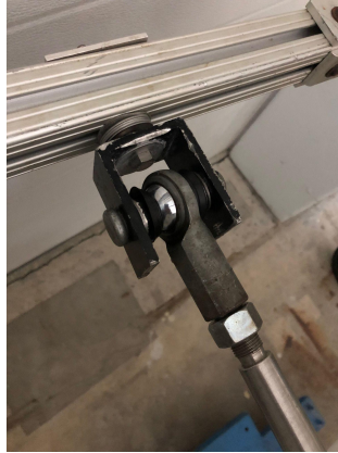
Figure 8: The ball joint rod end pin connection at the top of the piston shaft, connected to the crossmember of the gallows.
