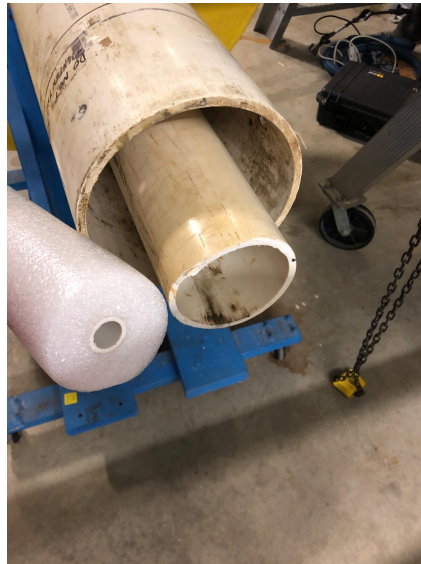
Figure 14: Shows the final pre-fabricated foam noodle used in the final design.
