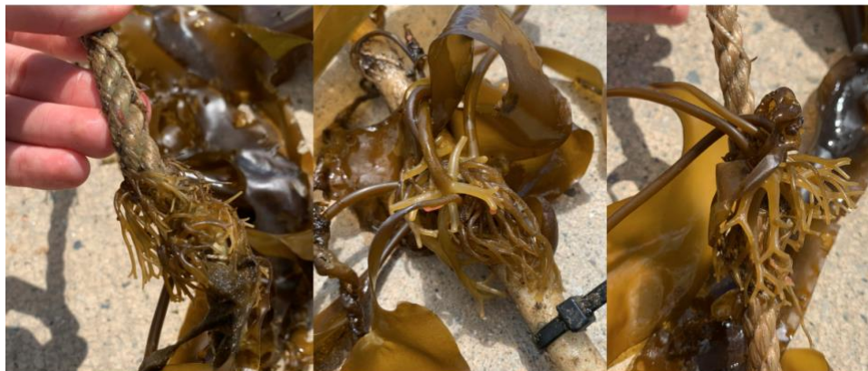
Figure 8: Comparing the kelp holdfast attachment at 4-week growth between polypropylene (left), composite (middle), and nylon (right)
