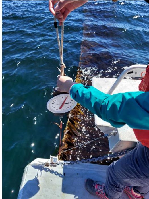
Figure 9. Holdfast attachment strength test set-up
