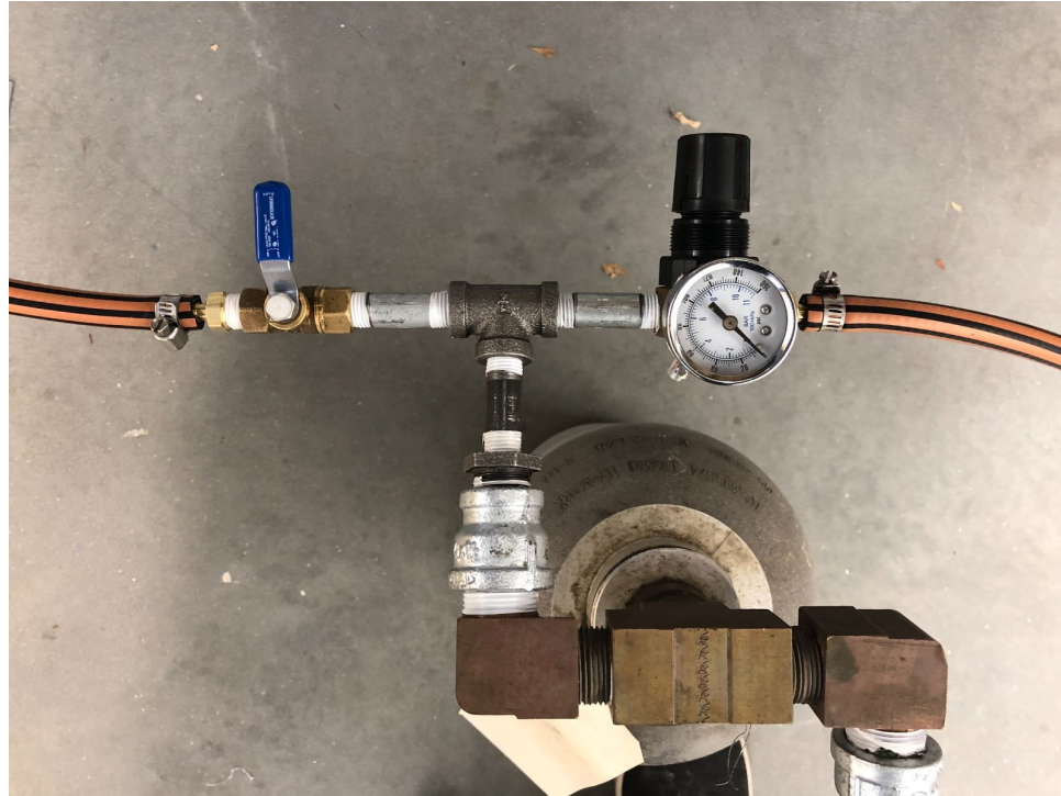
Figure 8: The pneumatic system for the experimental setup. The bottom right is a connection to the building air supply.
