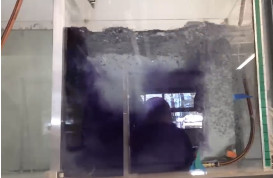
Figure 13: Image taken from video of circulation current formed due to the pressure drop induced by the bubble screen.
