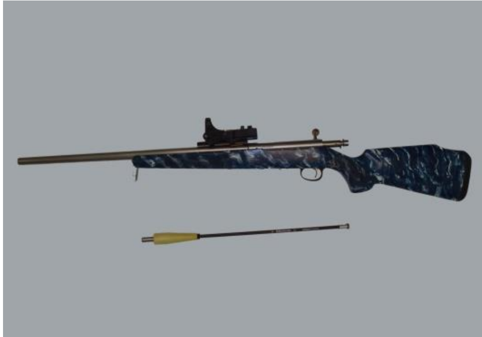
Figure 1. Modified rifle and dart used for remote biopsy sampling during the Natural Resource Damage Assessment of the MSC252 Deepwater Horizon Oil Spill.
