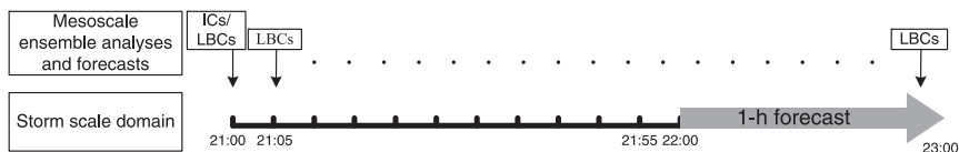
FIG. 7. Schematics of data assimilation experiment configuration. The radar data assimilation adopts the 5-min cycling, driven by the mesoscale analyses and forecasts. The 1-h forecast is then initialized by the analysis at 2200 UTC after 1-h assimilation.
