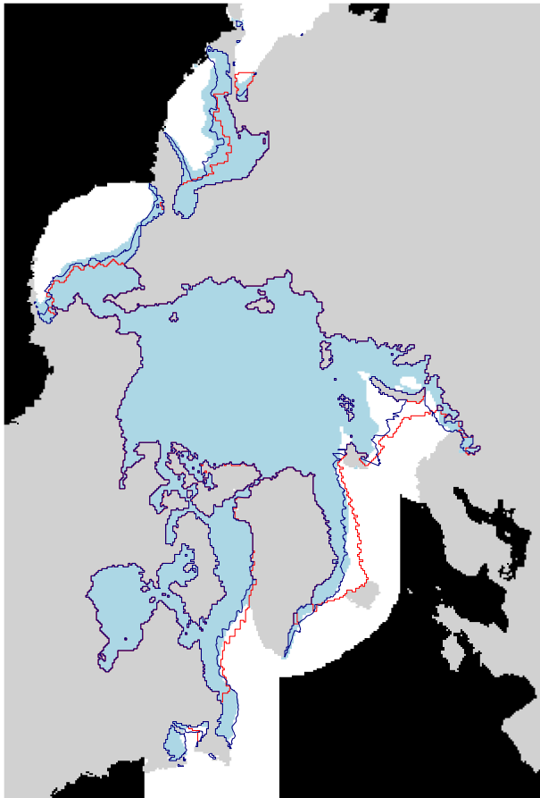
FIG. 1. Predictions for the 15% sea ice concentration contour obtained from the GFDL model with a 4-month lead time (red) and bias corrected using contour shifting (navy blue) for February 2012. The observed sea ice region is plotted in light blue. The black regions are part of the “nonregional ocean” in the ocean mask described in section 2a and are excluded in this analysis. The remaining white area represents grid boxes with sea ice concentration less than 15%.
