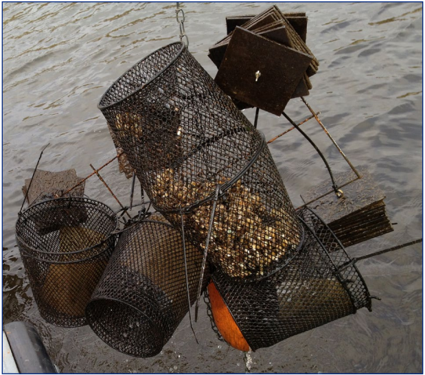
Figure 4. Caged mussels, passive samplers and Hester Dendys being retrieved after deployment for 6 weeks in Manistique River AOC.
