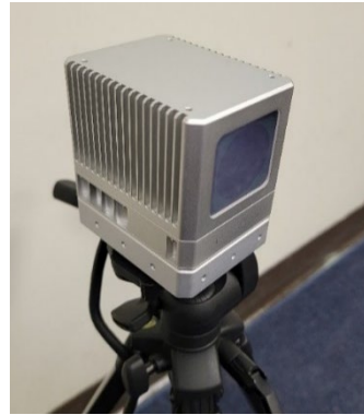
Figure 2. Livox® Mid-40 as mounted on a camera tripod.
