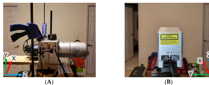
Figure 4. Orientation of (A) the Velodyne ® HDL-32E and (B) Livox ® Mid-40 during indoor data collection. The scanner orientations shown here were used for all data collection (indoor and outdoor) throughout the duration of this study.
