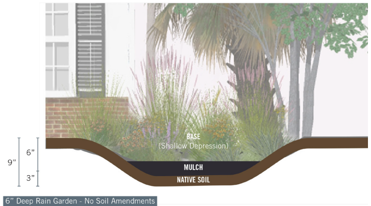
Figure 4: Rain garden cross section detail
