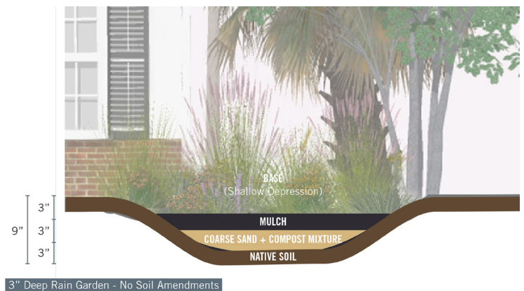
Figure 5: Rain garden cross section detail with soil amendments
