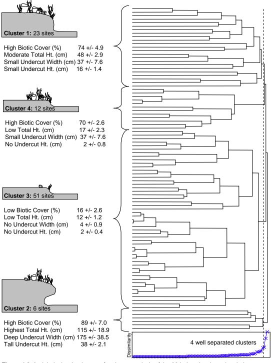
**Figure 4.8.** At right is the dendrogram for cluster analysis of the 92 ledge sites based on ledge measurements. The scree plot at the bottom indicates that there are four well separated clusters. Descriptive and quantitative characteristics (mean +/- SE) typical of ledges within each cluster along with a cross-sectional cartoon are noted at left.
