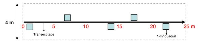
**Figure 2.1.** Schematic representation of the placement of the 1-m²-quadrat along a 25-m transect tape during fish and benthic substrate surveys at GRNMS. Broken line represents the total area surveyed (100 m²).
