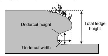
**Figure 2.2.** Schematic representation of the physical ledge dimensions measured during benthic surveys.
